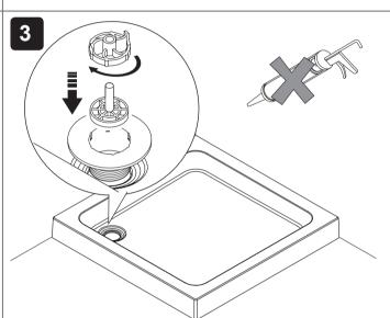
Fit the waste, as per the instructions supplied with the waste. Note! Do Not Use silicone sealant
