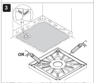
Install the shower tray on a bed of sand and cement or silicone
