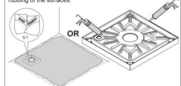
Install the shower tray on a bed of sand and cement or silicone sealant.
