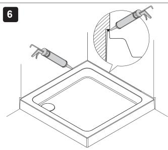
Apply silicone sealant in accordance with the manufacturer's instructions to seal the shower tray to the wall.
