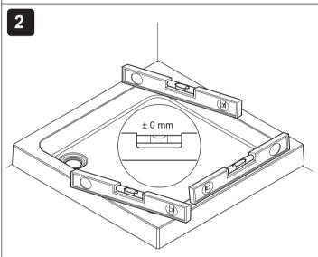
Place the shower tray on a flat surface and using a spirit level check that it is straight and flat and that the shower cubicle will sit on its surface correctly when fitted.
