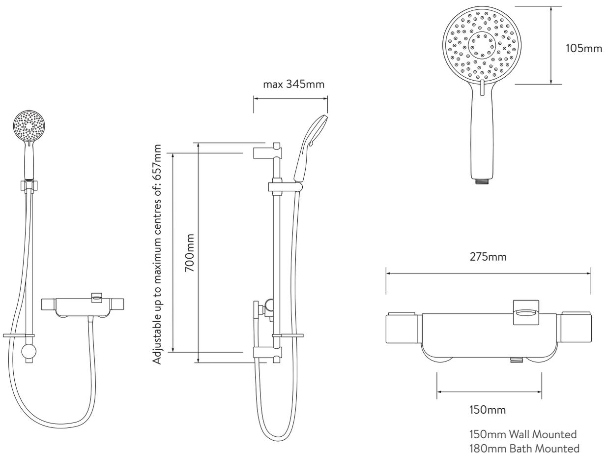
\*Pipe centres can be adjusted between 130mm-170mm using supplied elbows
