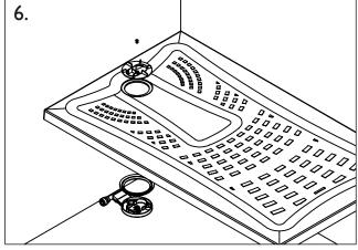
Assemble the shallow waste to the tray using the screw provided. Ensure the seal is positioned correctly and do not over tighten the screw. Ensure the waste is assembled correctly, incorrect alignment or assembly may result in a leak.
