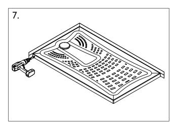
With reference to page 5 (Fig1) determine the pipe exit point and drill a hole in the side of the tray. This should be a minimum 16mm diameter to allow the 15mm waste pipe to pass through the side wall of the shower tray.
