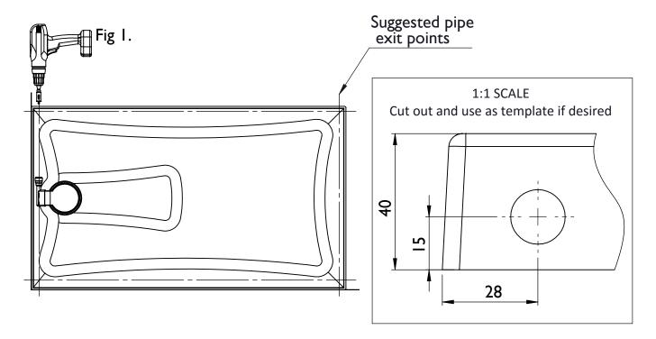
The tray design allows for 15mm pipe-work to be concealed around the underside perimeter of the tray. See suggested pipe-work routes and exit points. When the desired exit point has been established the side of the shower tray will need to be carefully drilled with a 16mm hole saw or similar.
