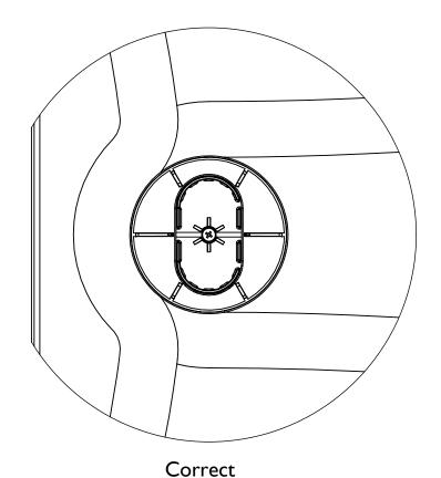
The waste outlet must be aligned as shown in this illustration.
