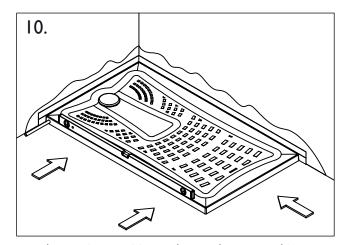
Put the tray into position and press the up-stand into the tile adhesive ensuring there are no air gaps. Check the tray is level on all four sides. Allow 24 hours before exposing to water.
