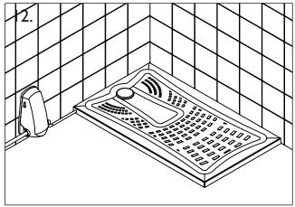
Fit the pump and connect up to the tray pipe-work. Ensure that the pipe-work is not under strain when connected.
