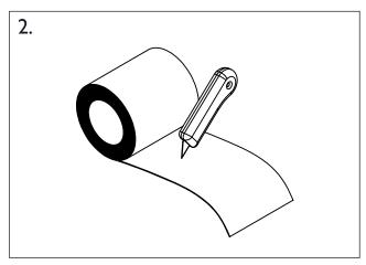
Measure and cut the required length of fabric tile up-stand.
