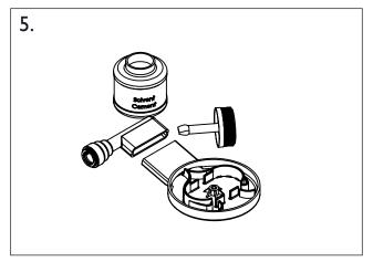
The outlet pipe needs to be bonded to the waste using solvent cement to ensure a watertight seal. Both components will need to have solvent weld applied to them.
