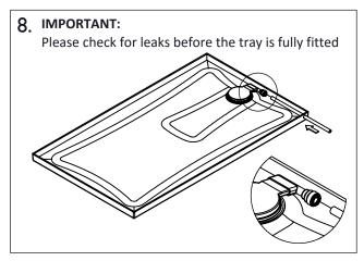
Feed the pipe through the drilled hole and connect to the waste pipe outlet, the other end will connect to the pump once the tray installation is complete. We recommend using copper tube.
