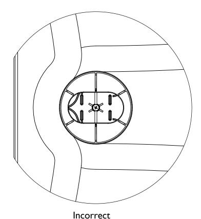
If the waste is assembled as shown here it will not tighten correctly and result in a leak. Under normal circumstances it should not be possible to assemble in this manner.
