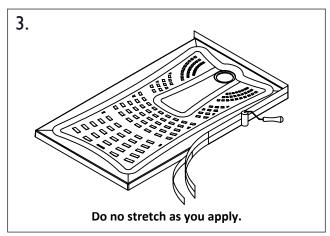
First remove of release paper. Carefully position against the tray and press firmly into place ensuring there are no bubbles or creases.
