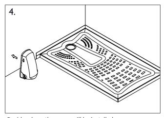
Decide where the pump will be installed. This will determine the waste outlet orientation in the next stage.
