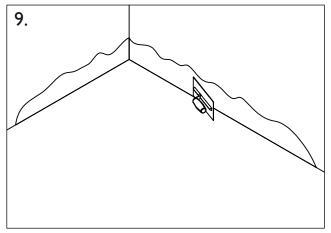
Apply tile adhesive to the wall ready for the tile up-stand. If the floor is not level this may be corrected by bedding down on sand and cement or tile adhesive.
